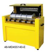
Stainless steel drums are rotating at a speed of  $100 \pm 5$  r.p.m. The Micro-Deval is supplied complete with control panel fitted with a digital automatic revolutions counter. Also stainless drums and stainless steel spheres are suplied together with machine .
